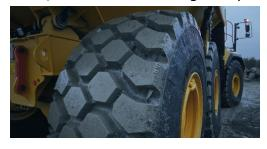
to an innovative tread, these tires offer long life even during the most intensive cycles thanks to a tread depth and a higher volume of rubber. What's more, the natural rubber used in the design of the MICHELIN XTRA DEFEND 33.25 R 29 offers reduced heat emissions in order to meet users' best productivity levels.
